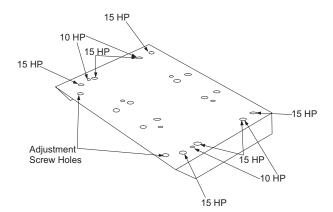
FIGURE 3 - LB600 MOTOR MOUNT PLATE
